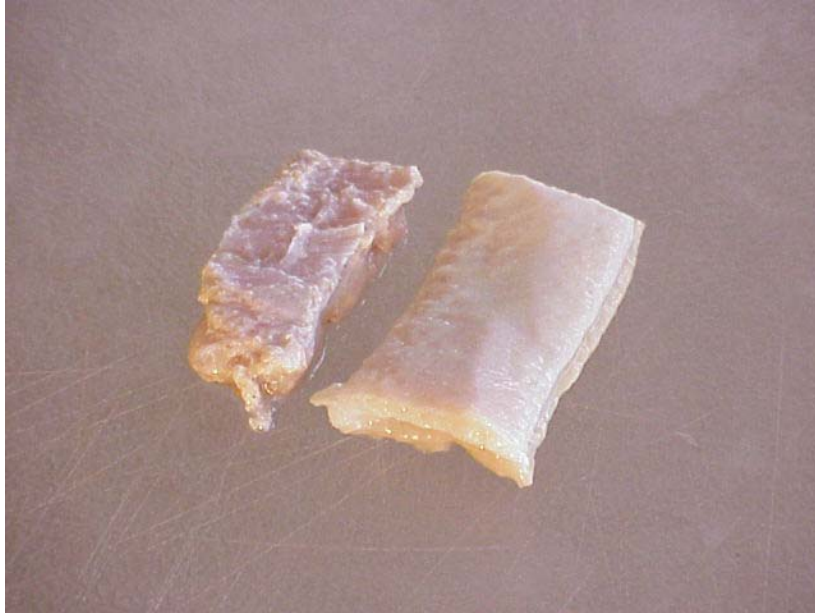
SADO vs. ALKDO Tests on Pigskin Sample on Left was exposed to SADO Sample on the right was exposed to ALKDO
